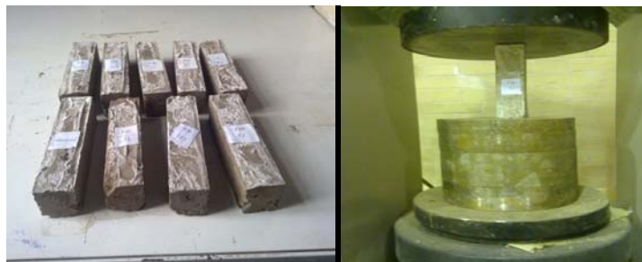
Figure 2. The mixed soil with fibers samples and testing method in this research
